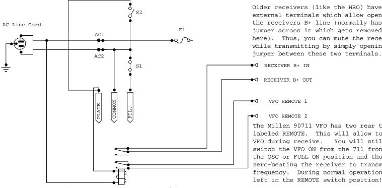
Dowkey 110VAC Antenna Relay with DPDT external contacts. RF relay connections are not shown here! Shown in Receive state (PLATE switch S2 on 90281 PS is OFF).
