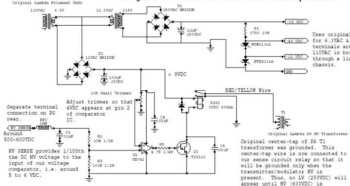
Uses original PS terminals labeled for 6.3VAC & 110VAC. Those terminals are no longer used. The 110VAC is brought in directly through a linecord into the rear chassis.
