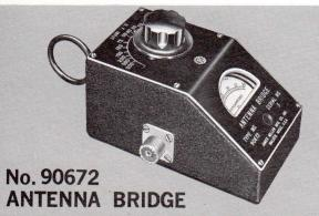
The 90672 Antenna Bridge is an r-f bridge which uses a Grid Dip Meter as a source of signal. It is a sensitive bridge for measuring impedance in the range of 5 to 500 ohms for unbalanced impedances and 20 to 2000 ohms for balanced input (using baluns) at radio frequencies up to 140 MC. Baluns available for measurement of balanced loads.
